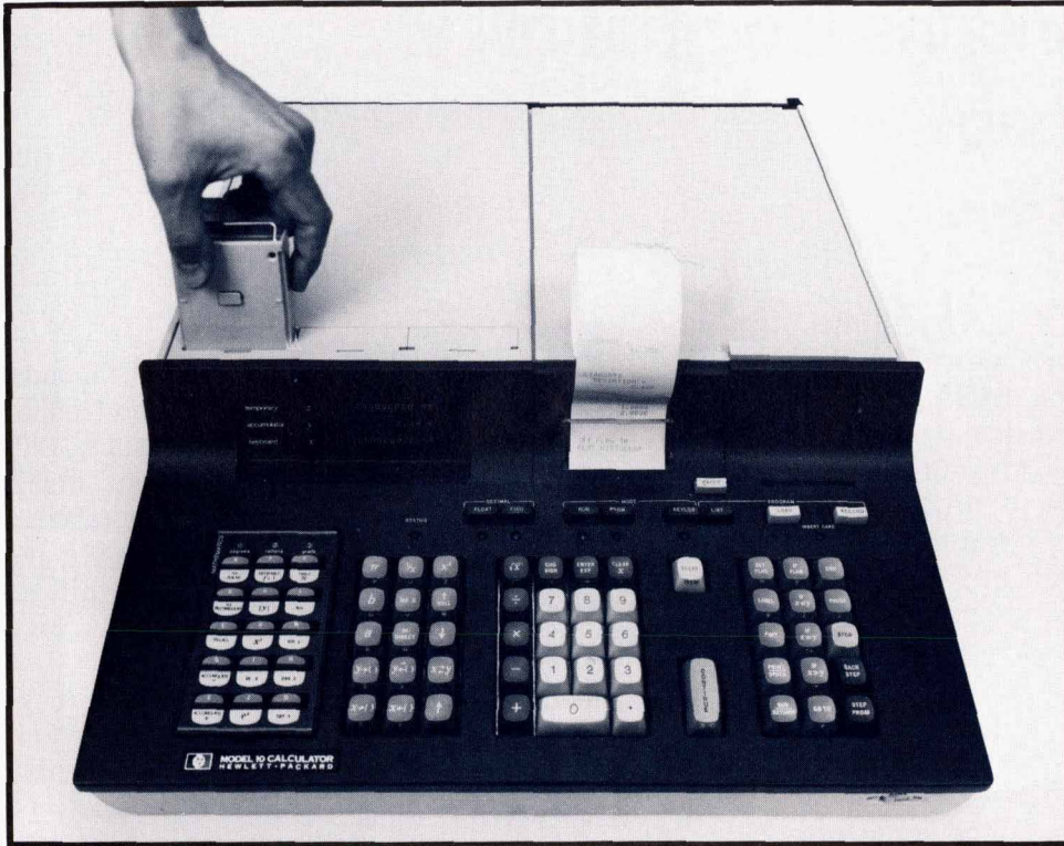
Fig. 1. Model 10 of the 9800 Series has all the capabilities of previous HP programmable calculators, plus many others. New features are the LED display, a larger internally expandable memory, decimal and indirect addressing, arithmetic operations into or from all data registers, and optional plug-in function blocks to define the lefthand keyblock and other auxiliary functions.
