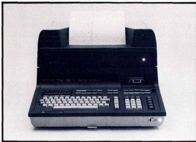
Fig. 2. Model 9866A Thermal Line Printer is the primary output peripheral for Model 30.
